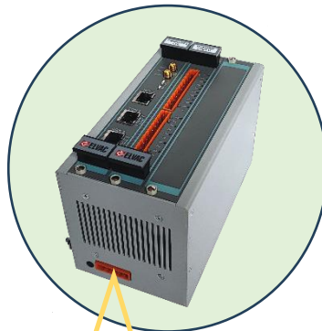
Power supply is integrated on backplane
